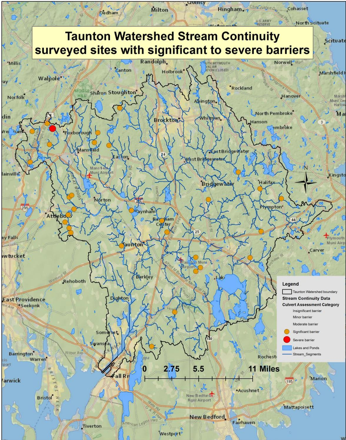
**Figure 17:** Locations of Crossings ranked as Severe and Significant Barriers to Aquatic Passage
